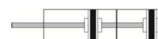
OPTION TA1 ÷ TA4 TANDEM VERSIONS TA1 = PISTON RODS COUPLED TA2 = PISTON RODS INDEPENDENT TA3 = BACKTOBACK TA4 = FRONTTOFRONT
