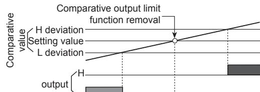
※After supplying power, there is no comparative output of L deviation (■).
