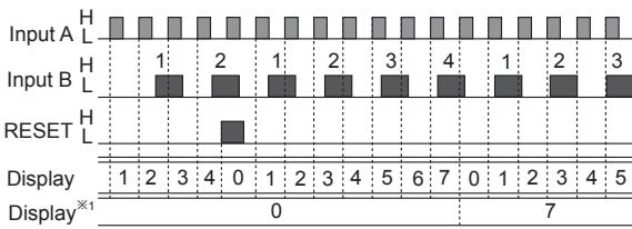
※1: When the display cycle[d1 5PL] setting is OFF, it will maintain the quantity of input A until the value of input B reaches the setting value B[COUNT.b].
