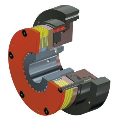
MAXITORQ<sup>®</sup> Model AFS units apply braking torque when the hydraulic or air pressure is removed from the piston chamber, which can occur intentionally or when there is a loss of pressure. When pressure is removed from the piston chamber compression springs clamp the MAXITORQ<sup>®</sup> multiple friction discs between the pressure plate and the stationary end plate, which results in a consistent holding force.
