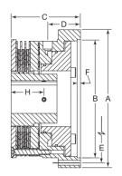
An optional protective cover is available to prevent debris or moisture from entering the friction disc surfaces, which is often helpful for exterior applications or dusty environments.
