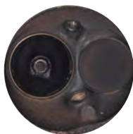
Cylinder head before P.i. treatment.
