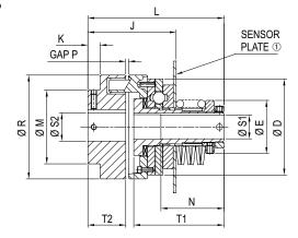
① See page 14, Table 20 for dimensions and movement on disengagement. NOTE: Temperature range of elastomer bushing is -30°C to 80°C (-22°F to 176°F).
