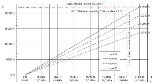
$\mu$  = Nominal friction between brake pad material and brake disc.
