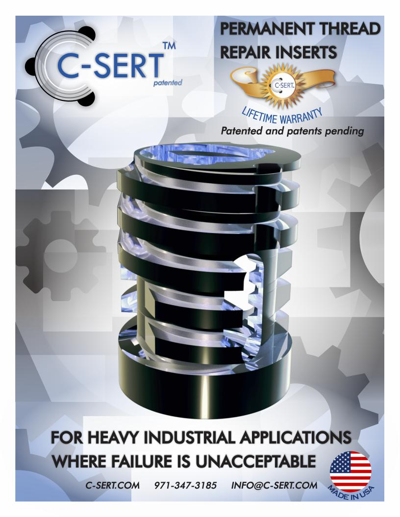
**Advantages** TOOL STEEL CONSTRUCTION \* Benefit: Can't wear out **LEFT-HANDED EXTERNAL THREADS** \* Benefit: No back-out with stuck bolts **SELF-TAPPING** ❖ Benefit: Fast **SELF-ALIGNING** \* Benefit: Goes in straight **BUILT-IN DIE** \* Benefit: Trues up bad bolts Thread-chasing die Female drive slots S-7 tool steel Internal R-H threads Left-handed engagement threads **ACME threads** Flute Chip relief Cutting slots and teeth Integral pilot
