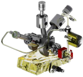
Forced lubrication with low pressure gear pump
