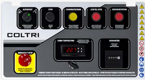
Compressor control and automatic condensate drain system
