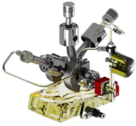
Forced lubrication with low pressure gear pump
