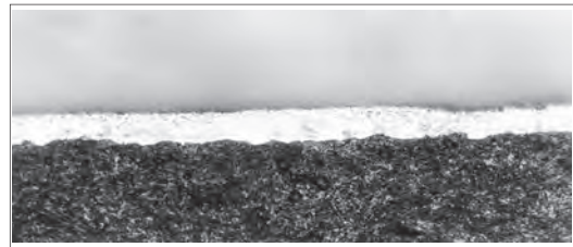
The white layer is a layer produced by DHA treatment, and the black grains visible in the layer are chromium carbide
