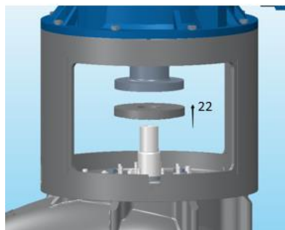
Remove the seal cover (22) with the stationary ring of the mechanical seal.
