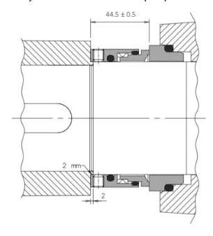
Also make sure that the electric motor is with locked bearing in the drive end – i.e. there must not be forced axial stroke of the electric motor.
