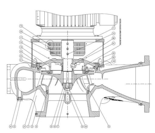
Pump casing 1 2 Pipe plug 3 Pipe plug Sealing ring 4 5 Impeller 6 Cap nut 7 Spring washer Inlet cone 8 9 Sunk key Mech. shaft seal 10 17 Shaft 18 Rear cover 20 Motor bracket 21 O-ring 22 Set screw 23 Washer 24 Stud 27 Seal ring 2 28 Guard 61 Plug Set screw 64 71 Set screw 73 Pointed screw 75 **INSEX-screw**
