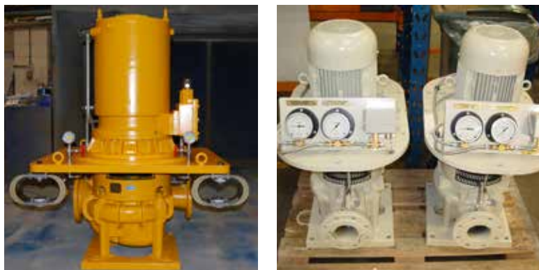
Shock Rated Engine Room Pump
