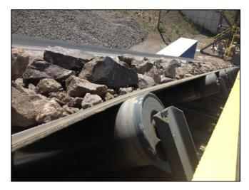
Adjustments for belt alignment on the carrying side should begin at the tail pulley. If necessary, the angle of idler with center line can be changed slightly. As on the return side, the belt will shift toward the side where it first touches the idler rolls.
