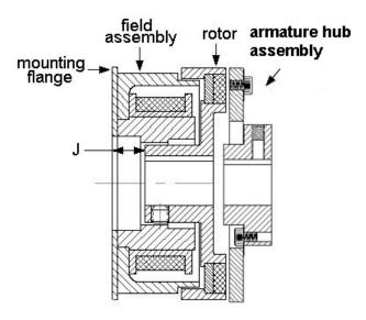
FO series power-on clutches are used to couple two inline shafts. The field assembly is mounted to a bulkhead that is perpendicular to the clutch shaft and then the rotor is assembled to the shaft. Typical FO clutch installations provide a coupling between the drive and the driven shaft.
