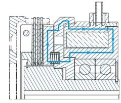
Radial magnetic flux path provides maximum torque throughout life of clutch.
