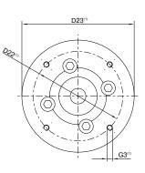
Drawing corresponds to a HLAE070 / 1-stage / output shaft with feather key / 11 mm clamping system / motor adaptation - one part / B5 flange type motor
