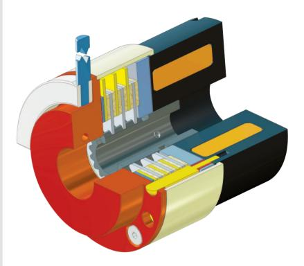
MAXITORQ® Model HTB brakes are a cost-effective solution when exceptionally high torque in an extremely small package is required. The HTB brake is released when power is applied to the brake coil. When power to the brake coil is removed, braking torque is applied.
