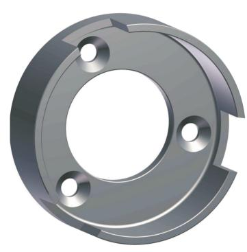
Carlyle Johnson Maxitorq® internal flange type driving cups are designed to provide an economical means of adapting the clutch or brake to various types of driven or driving members with a pulley, fly wheel, sprocket, gear, or sheave by means of flathead screws. Cups are hardened for long life and durability. The internal flange drive cup has a smaller outside diameter and a lower inertia, then the ring type driving cup.
