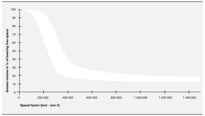
The area marked in white indicates the grease fill as a function of the speed factor
