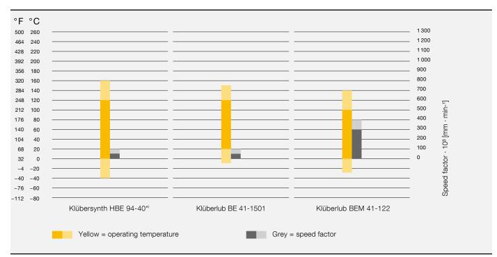
The darker areas are the target if lifetime rolling bearing lubrication is required.
