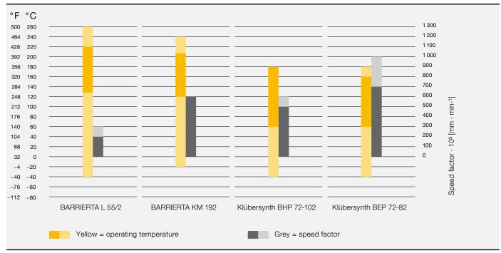
The darker areas are the target if lifetime rolling bearing lubrication is required.
