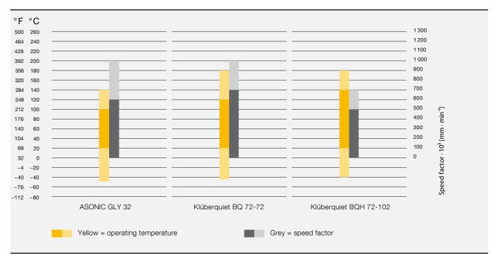
The operating temperature range and the maximum speed factor  $n \cdot d_m$  can be read from the diagram. The darker areas are the target if lifetime lubrication is required.
