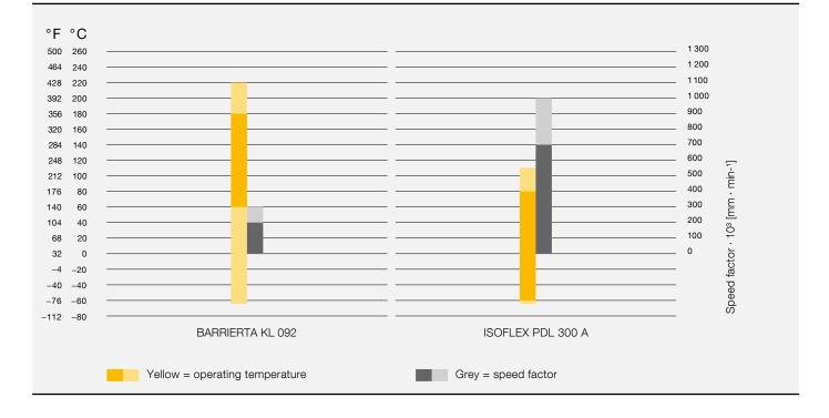
BARRIERTA KL 092 and ISOFLEX PDL 300 A are lubricating greases which are particularly suitable for low-temperature applications. Please contact our technical consultants for an estimation of the grease service life in your application.
