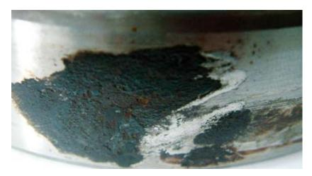
Fretting corrosion on the outer ring
