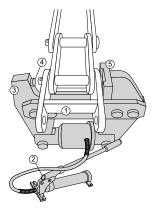
Part Identification 1-Spacer Gage (Rectangular) 2-Relief Valve 3-Force Arm 4-Ram 5-Support Plate
