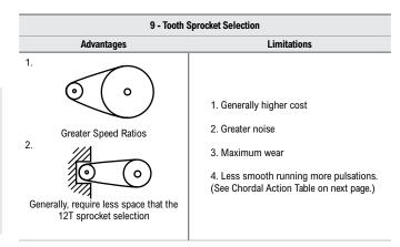
Select a 15T Sprocket where long centers are necessary and space is not a limiting factor, where maximum speed ratios are not required, or where quiet operation is desired.
