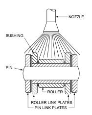
When manually lubricating, the oil should be directed between adjacent outer and inner sidebars (for the joint) and between inner sidebar and roller face (for rollerbushing lubrication). For best results, clean chain and sprocket periodically.
