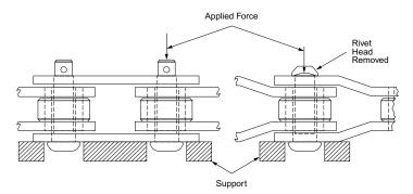
Figure 2 - Type I Connector Removal
