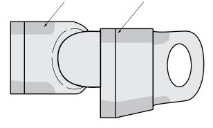
Selectively Induction Hardened sidebars can be ordered to give greater resistance to abrasive sliding wear, thus providing greater sidebar life.
