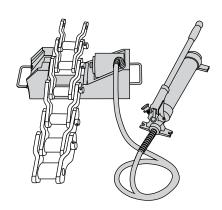
Easy-to-use Drivemaster assembly tool reduces down-time, maintains interference fit and eliminates cumbersome assembly/disassembly methods.
