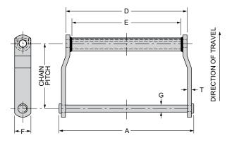
Rexnord Wide Series chains are specially designed for loads and operating conditions imposed by drag conveyor service. As with our Narrow Series, many material and configuration options are available.
