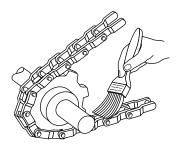
The effectiveness of any lubrication method will vary with the amount of lubricant used and the frequency of application. Ideally, a lubricant film should be maintained between working parts.
