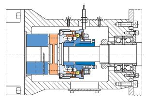
The EAS<sup>®</sup>-compact<sup>®</sup> with a backlash-free, torsionally flexible and vibration-damping shaft coupling for the connection of two shafts. The coupling compensates for axial, radial and angular shaft misalignments.
