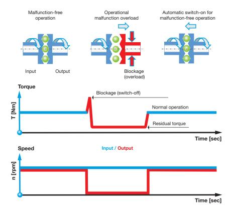
Example 2: Torque and speed paths of a load separating ratchetting torque limiter
