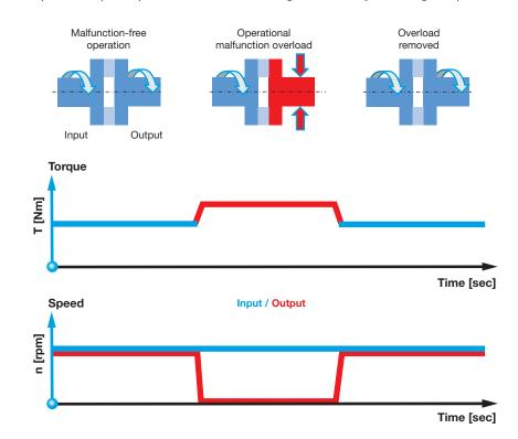
Example 1: Torque and speed paths of a load holding frictionally-locking torque limiter
