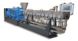
The operating conditions for extruders place maximum demands on drive systems: Only special, optimised clutches for torque limitation, such as the EAS<sup>®</sup>-dutytorque, guarantee reliable protection in case of overload.
