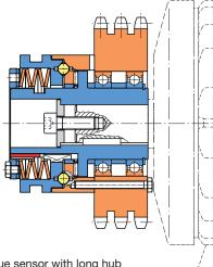
EAS®-torque sensor with long hub and mounted triple chain sprocket
