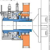
EAS<sup>®</sup>-Sp clutch mounted onto the shaft end: The clutch is axially secured via a cone bushing and allows a backlash-free torque connection from shaft to hub.
