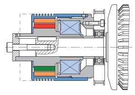
The clutch is secured directly onto the motor shaft and the pulley is bearing-mounted separately using the deep groove ball bearing (used as a clutch for torque limitation).
