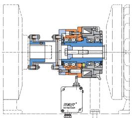
$EAS^{\circ}$ -Sm with torsionally rigid flexible all-steel coupling positioned between the motor and the gearbox. When the clutch disengages, the armature disk moves axially and operates the limit switch.
