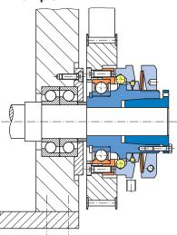
EAS<sup>®</sup>-compact<sup>®</sup>-F with a short hub: The clutch interrupts the transmission between the motor and the toothed belt pulley on overload and remains disengaged.
