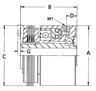
Important: When the Model AHA clutch or brake is operated with compressed air, it is necessary to incorporate an air filter and lubricator in the supply line near the clutch or brake to ensure clean air and sufficient lubrication to the piston seals.
