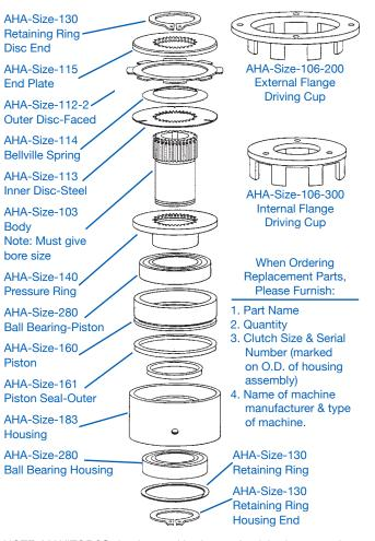
NOTE: MAXITORQ® clutches and brakes as furnished can run dry or in oil. We specifically recommend Series A oils when operating wet. If extreme pressure additives that would reduce clutch torque are utilized, please contact the factory for recommendations.
