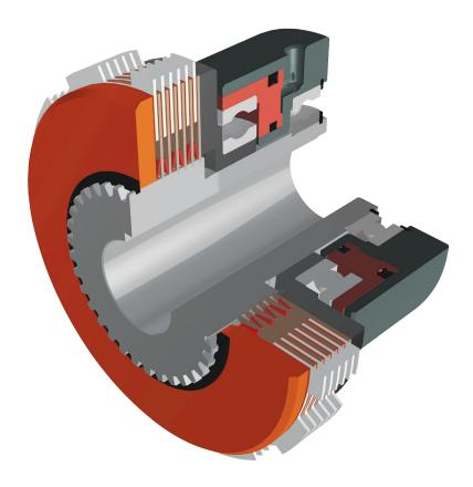
AHA model MAXITORQ® multiple disc air/hydraulic clutches and brakes provide high-performance operation, delivering more than 10 times the torque of single disc air/hydraulic units of the same package size. Featuring the patented MAXITORQ® floating disc principle, these clutches and brakes ensure minimal resultant heat when in neutral, fast disengagement and low neutral drag. Customization is available to meet specific operational needs, including wet or dry applications.
