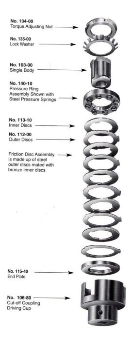
**NOTE:** Maxitorq® Torque Limters as furnished can run dry or in oil. We specifically recommend Series A oils. If high gear loading or worm and wheels are adjacent to the clutch and indicate extreme pressure additives that would reduce clutch torque, please contact the factory for recommendations.
