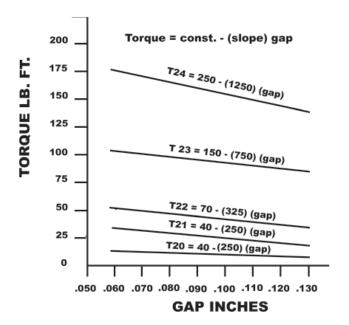
Spacing or "gap" between pressure ring and facing bronze disc is a meassure of torque.
