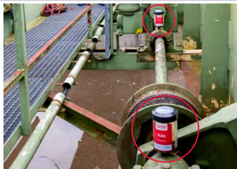
Roller bearing lubrication on a scraper
