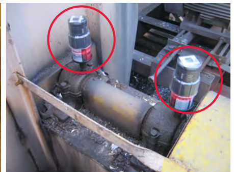
Lubrication of a fan drive shaft bearing
