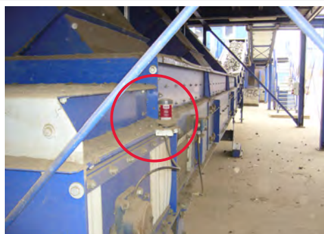
Flange bearing lubrication on a conveyor
