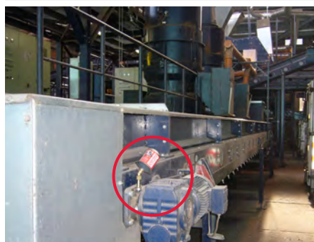
Flange bearing lubrication on a conveyor
