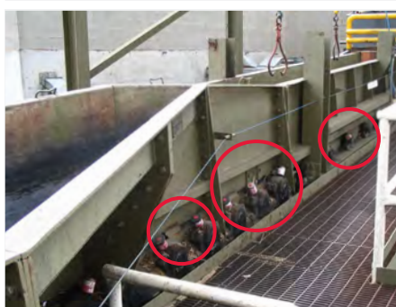
Bearing lubrication on the tree sorting system
