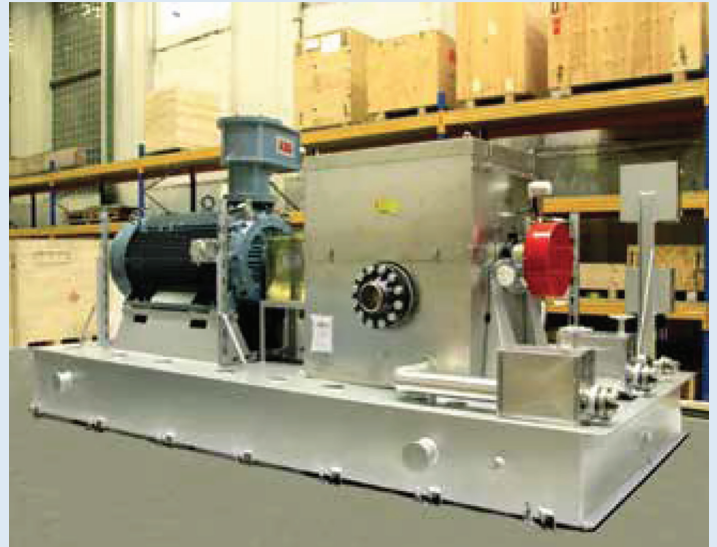
Pre-heated system arrangement or several types of steam Jacket options (photo) available.
