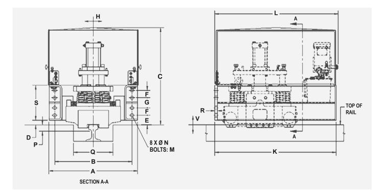
V Vertical Rail Deviation (Float) ±25mm relative to Rail Clamp enclosure at full rated capacity.
