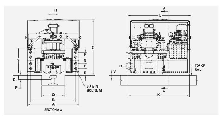
1V Vertical Rail Deviation (Float) ±25mm relative to Rail Clamp enclosure at full rated capacity.
