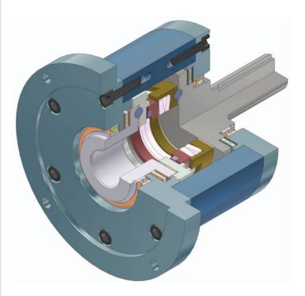
MAXITORQ® Model MTL TORQ-LOK® is a patented, one way, bi-directional clutch that permits the transmission of torque from the input shaft to the output shaft in either rotational direction. With its unique design, the MTL does not allow the output shaft to backdrive the input shaft.
