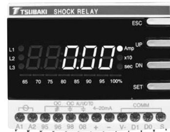
All-in-one type (built-in current transformer)
