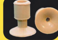
3121 MIEHLE CS and other feeders. For heavy stock or sheet metal. 1-7/8" high, 1-9/16" across. Fits 3/4" OD tube or 1/2" pipe.
