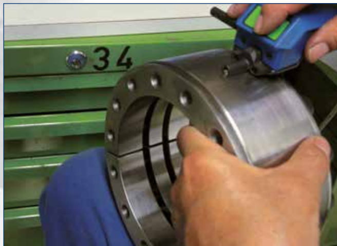
Rauheitsmessung / Surface roughness measurement
