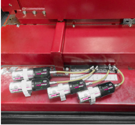
Four simalube IMPULSE connect pressure boosters lubricate the linear guides of a CNC machine by means of hose connections. Each IMPULSE can be controlled and configured individually with the simatec app.
