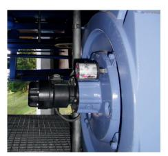
The drive of a gondola lift on the mountain station is lubricated continuously with a 60 ml lubricator.
