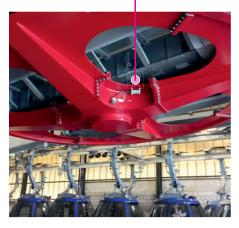
In the valley station, the deflection roller of a chairlift is lubricated with two simalube 250 ml lubricators.
