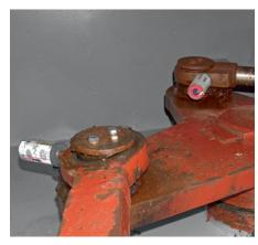
The steering wheel is lubricated with two  $125\,\mathrm{ml}$  lubricators.
