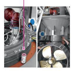
A simalube 125 ml seals the thruster so that no water can enter.
