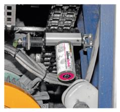
The simalube lubricator continuously oils chains, even in tight spaces. Additionally, the brush cleans the chain.
